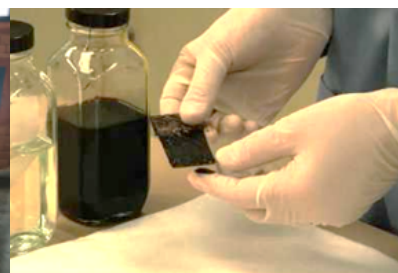
Chemical Resistance Tests
